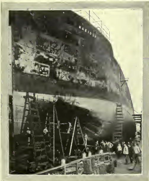
REPAIRING A SHIP DAMAGED BY A MINE.
