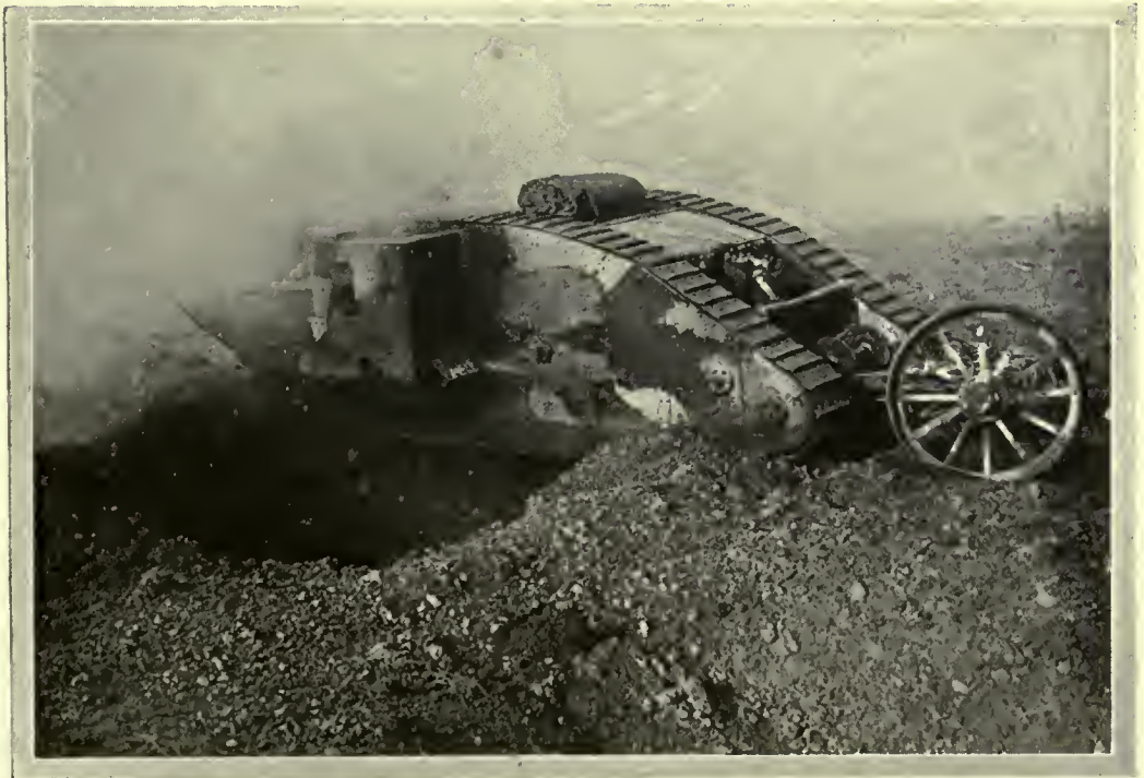
Fig. 6. A BRITISH "TANK" IN ACTION CROSSING A SHELL-CRATER.
